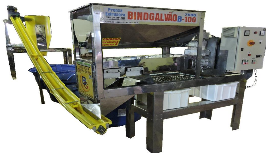
Figure 1. Image of the cold extruder press which is extracting the oil and as a by-product produces the soybean meal. Source: www.bindgalvão.com.br .
